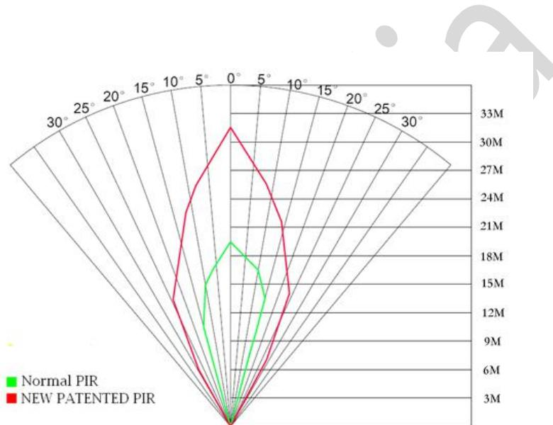
The PIR detection angle ( $\alpha$ ) is just smaller than the field of view (FOV) angle ( $\beta$ ). The advantage of this design is to reduce empty picture rate and capture most, if not all, motions.
