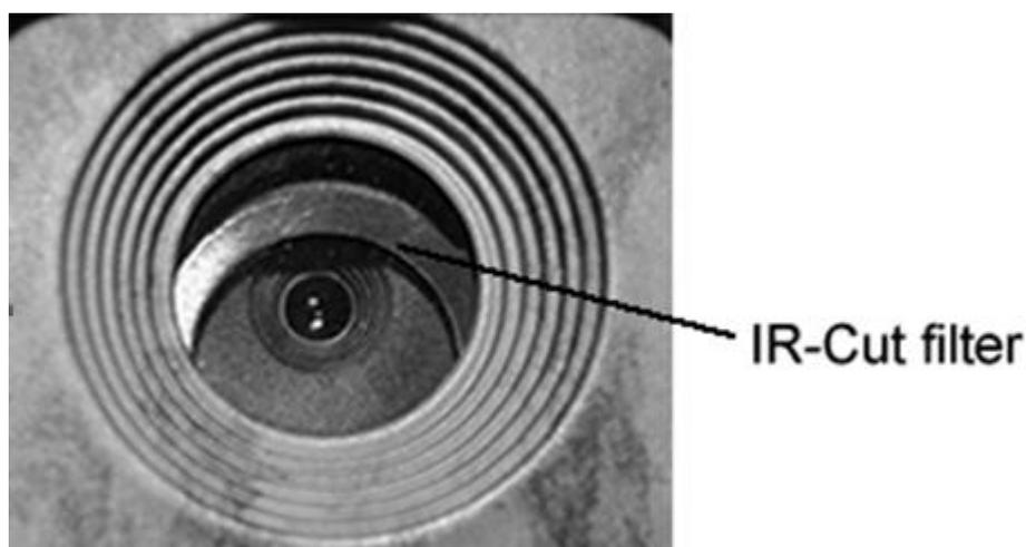
A: The camera is not broken. It's an IR-cut filter. When the camera is powered on, the IR-cut will be reset and cover the lens. Only when the camera is powered off, the IR-cut will be at a random place.
