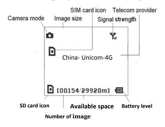
indicates the SIM card is recognized by the camera.
