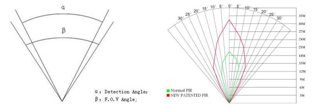
This camera has a new, patented design of the PIR. The new patented PIR's detection range can reach to 100ft (in good environments). The previous picture shows the compared detection zone between normal PIR and the new patented PIR.
